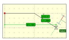
Precise coordinate specification of relative bar elements in the Cartesian and polar system.
