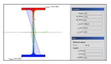
Gradient maps of normal, shear and reduced stresses in any sections of bars.
