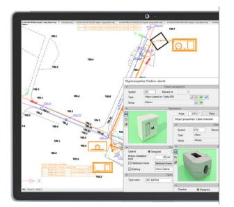
The ArCADia-TELECOMMUNICATION NETWORKS program enables the design of external telecommunications networks along the route: initial distribution frame (initial cable end: distribution frame, external cabinet, cable box) - telecommunication line route - end distribution frame (final cable ending of line: distribution frame, external cabinet, cable box, cable termination in a building), as well as any configuration of the network with its breakdown into selected components.
