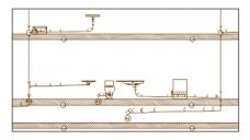
Automatic generation of developments: drain pipes, risers, approaches with accessories including fittings and sewage system devices.
