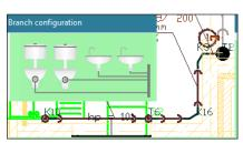
Drawing facilities allowing for a quick and easy way to create the connections of a number of outflows at the same time, depending on the connection method and the intended use of the fixture.
