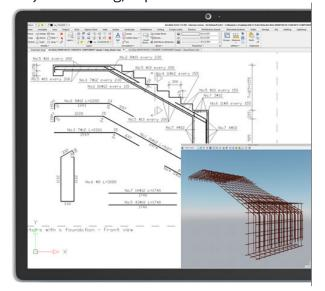
The module allows for object insertion of reinforced concrete elements that are parameterized in the Lisp script, as well as generating views and cross-sections automatically.
