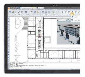
ArCADia-IFC RVT, in the new version of the ArCADia BIM system, changes the approach to IFC file reading by importing them without any conversion. This allows the model to be loaded more precisely together with all the data of any object for creating each building.
